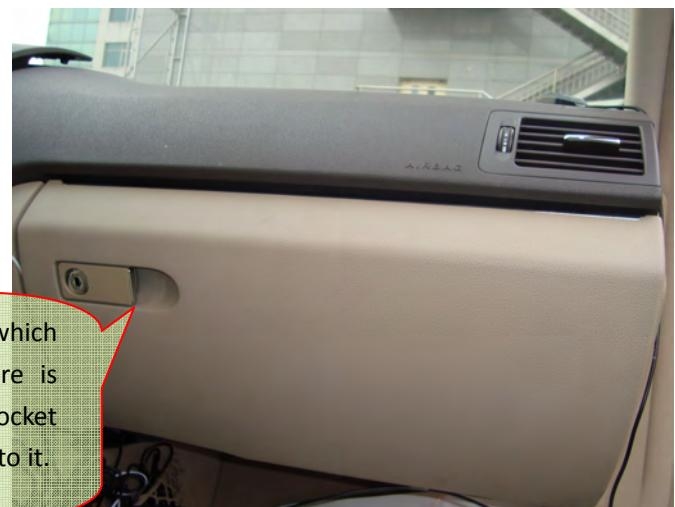
Open this drawer, then 4 screws can be seen, which will release the drawer when removed. There is enough space behind. Attention to the AUX socket should be paid, since there are wires connected to it.
