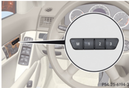
M Memory button 1, 2, 3 Memory position button
