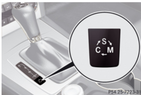
Program mode selector switch on C 63 AMG
