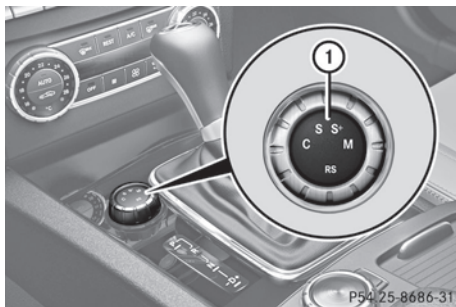
Drive program selector with manual drive program
