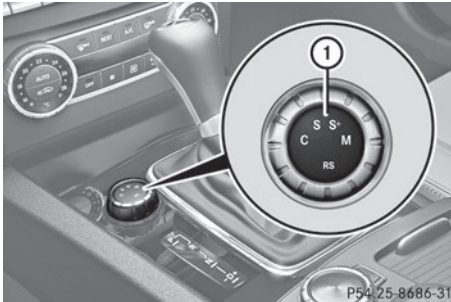
Drive program selector with manual drive program
