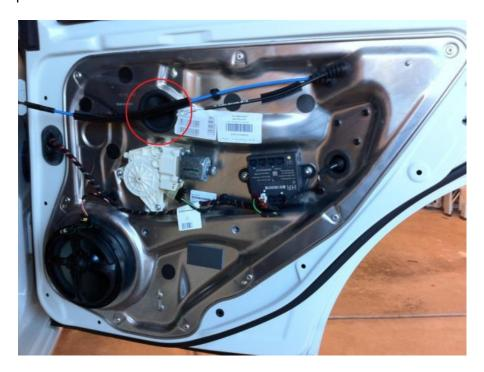
3. Lower the window until you see the clip securing the glass in place. Unscrew only until the tension is released.
