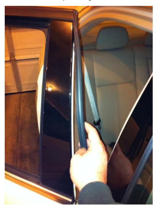
6. Pull the next seal up out of the door and away from the window frame. This seal servers as one of two guides for the glass.
