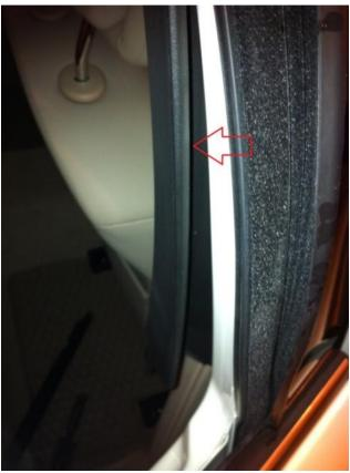
5. Pull the rubber seal out away from the edge of the door.
