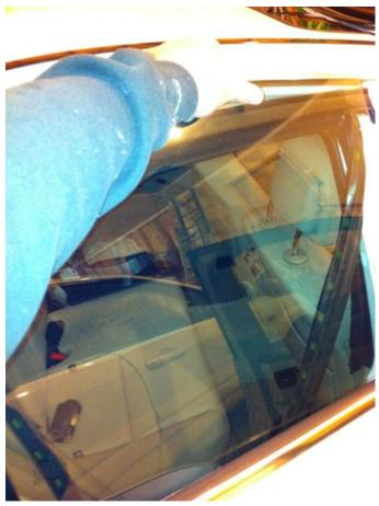
10. Once the old glass is removed you can install the new piece of glass in the reverse order. When the new glass is installed tighten the clip securing the glass to prevent it from moving. Be sure to allow room on each side of the glass for the rubber window guides. Forcing the rubber back down into the door in the proper place is a pain in the neck. Once they are back in place, operate the window and adjust the glass left or right accordingly so that it moves freely.
