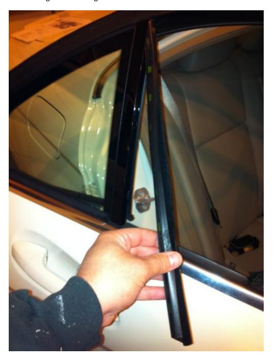
7. Repeat the same process on the other side pulling the seal up out of the door. This will expose the three screws indicated in the picture.
