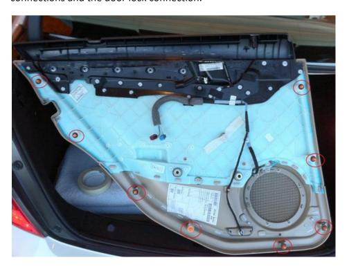
2. With the door panel removed, pull off the rubber cover indicated with the red circle in the picture below.
