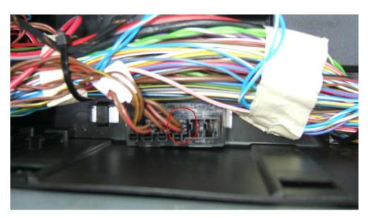
Next, feed the fuse wire and the longer end of the 2<sup>nd</sup> cable harness over the transmission tunnel to the drivers side. You may need to use a cable rod or coat hanger to feed it through. The picture below shows the cables having been routed through to the drivers side.
