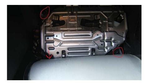
The picture below shows the back side of the footplate. The circle shows the grounding point which is used later and the square shows the position the CAN module is fixed to.
