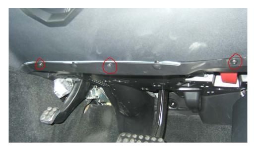
Now move to the passenger side and remove the same trim pieces except the part above the footwell and the carpet by simply untucking it from the trims and pulling it out. This exposes a foam pad which unclips from the bottom and behind that is the metal footplate.
