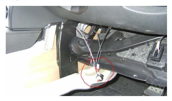
Now, on each end of the 2<sup>nd</sup> wiring harness there are 2 black connectors. One fits the connection on the door sills and the other fits the connection on the converters. Using the double sided tape, glue the converters in place. The instructions call for the converters to be fitted to the side of the cable duct but I chose to put them on a small empty section of the cable ducting itself. They are a nice tight fit and are held securely. See picture below.
