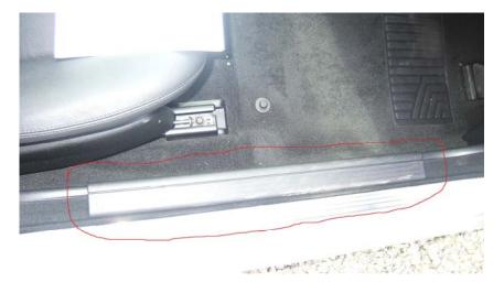
Next, remove the lower A pillar trims. These are clipped in place so pull them towards the centre of the car and then unclip them at the bottom. The drivers side trim has a section that attaches to a pin circled in the picture, the arrow points at the door seals which when pulled back expose the clips.
