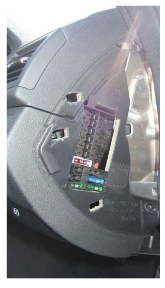
Now, some cars will not have the interior fuseboard and the fuse will need to be routed through to the fuseboard under the bonnet and connected there instead.
