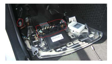
Next its time to install the CAN module. Take the module and completely cover the reverse side in double sided tape. Make sure the surface is clean first.
