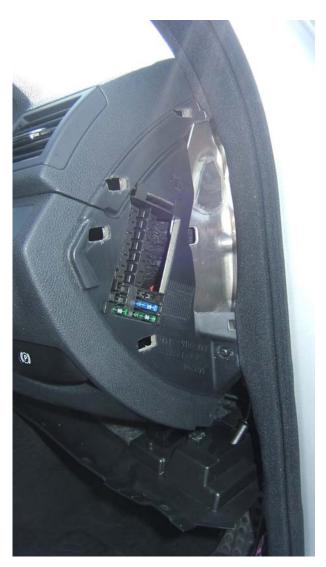
Next, remove the fuse from the connector and feed the cable up into the dashboard and through the hole where the fuseboard was. Clip the connector into slot 129 and put the fuse back in. See below for the finished article.
