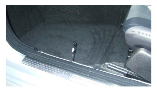
Now, at the drivers side you will have one cable left to fit which will have the fuse on it. This needs to be connected to the fuseboard. Pull out the cover on the side of the dashboard to reveal the fuseboard. The fuse board simply unclips and can be pulled out.
