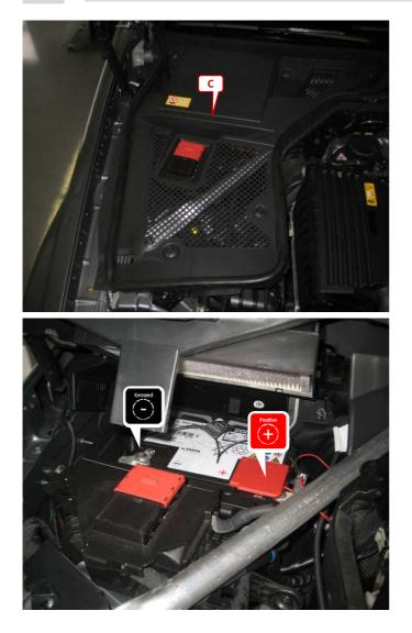
Open the cover (C) from the vehicle battery.
