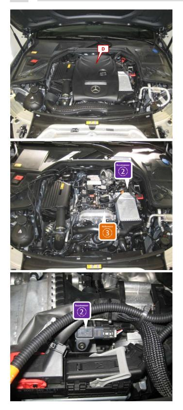
Open the engine hood and remove the engine cover (**D**).
