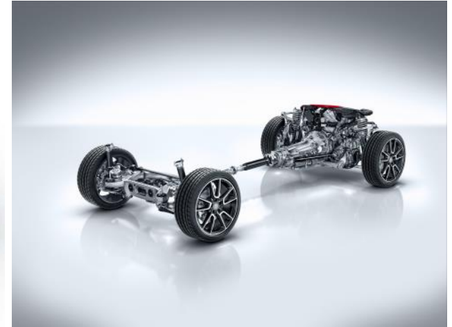
AMG Performance 4MATIC Torque Split – 33% Front / 67% Rear
