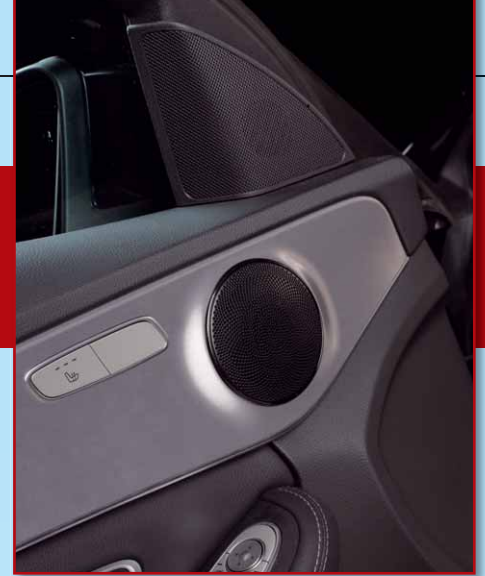
In our case, there are installation spots for a two-way compositystem in the front doors of the C-class
