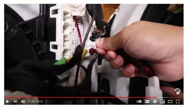
There are also these 4 connectors: 13, 14, 15 and 16. Connector 13 is left for 3D tweeter (I think so). Connector 16 goes to light tube. I do not know the function for connectors 14 and 15. ALL OF THEM ARE FEMALE CONNECTORS.
