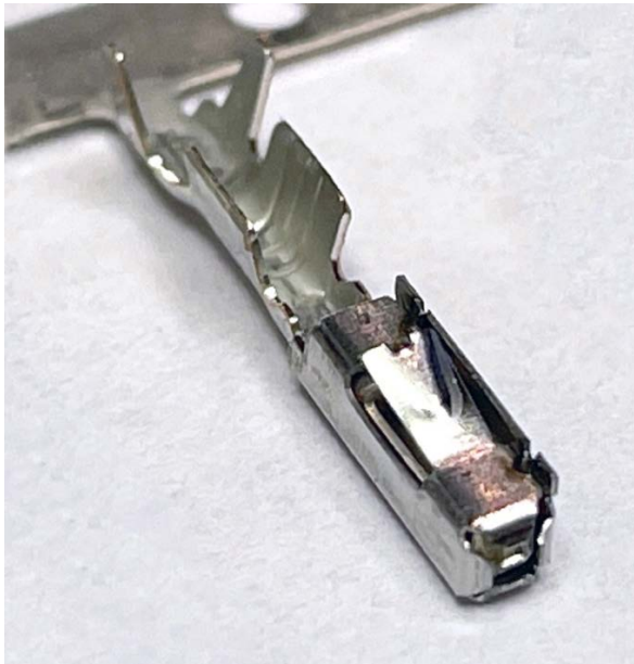
(Pin for the Taillight and the Rear SAM HL & HR)
