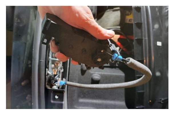
b) Attach the cable to the new motor (the cable should wrap around, and the blue piece should snap into place as shown)
