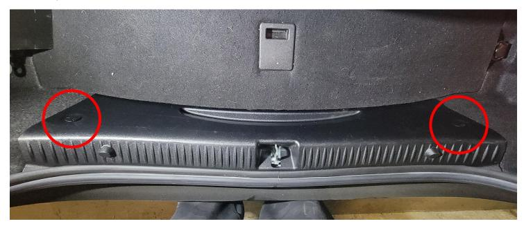
I found this to be the most difficult part. I pried the rivet a bit with the trim removal tool, once they were partially extracted, I used needlenose pliers to grab them and pull them out.
