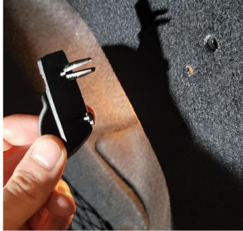
c) Pull back on trim to reveal motor unit. You may have to use a trim removal tool to pry it free.
