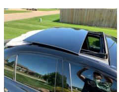
Step 2 – Remove the 2 Torx screws from the carriage located up under the glass. Repeat for the other side. Now slide the glass back about 6" to gain access to the clips.
