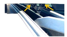
Step 3 – Remove the old/broken clips. If they are not broken, they may be cut out with a utility knife or oscillating tool.
