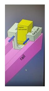
10- Once the bindings are in position in the cleats, lock them by pushing the 2 pins (use a pin-type tool to push the pins into position until they are flush with the face of the cleat)
