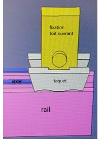
9- Exert slight pressure on the sunroof so that the fixings go down to the bottom of the cleat. (if necessary use a flat screwdriver to spread the cleat a little)
