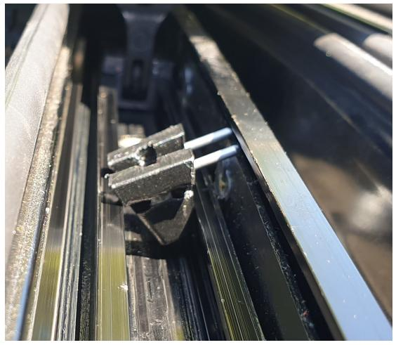
5- Press (lightly) the 2 upper sides of the cleat and rotate it (if the 2 locking pins bother you, remove them and reinsert them a few mm once the cleat is positioned)
