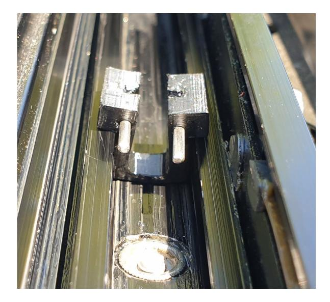
7- Slide the cleat under the sunroof mounting Repeat the operation for the other slider so that the sunroof mountings are both resting on the cleats
