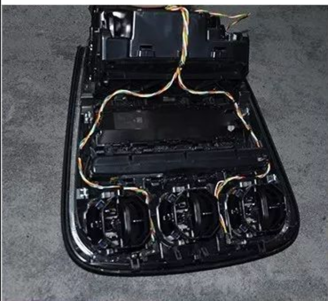
Slot in Center Console Light Tube and LED bulb
