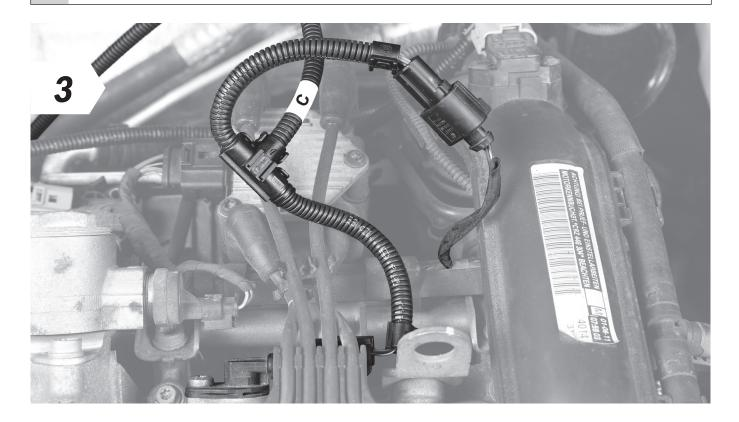
• Now connect the end of the RaceChip wiring harness marked "C" to the disconnected connector and the other end to the sensor.
