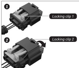
In the first step, the orange *locking clip* 1 is pulled out. Press the black *locking clip* 2, which functions as a lever for loosening the plug and pulling it out.
