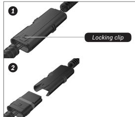
The plugs are locked into the connection sockets by means of a *locking clip*. Pull slightly the *locking clip* and pull the plug.
