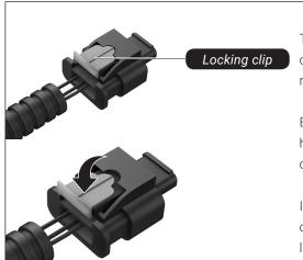
The first step involves pulling out the bright grey *locking clip*. Press down on the bright grey *locking clip*, which serves as a switch for releasing and removing the plug.
