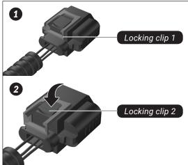
In the first step, the red *locking clip* 1 is pulled out. Press the black *locking clip* 2, which functions as a lever for loosening the plug and pulling it out.
