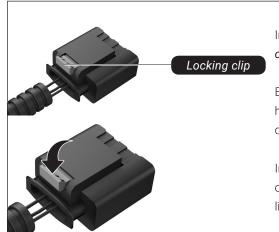
In the first step, the grey *locking clip* is pulled out. Press the grey *locking clip*, which functions as a lever for loosening the plug and pulling it out.
