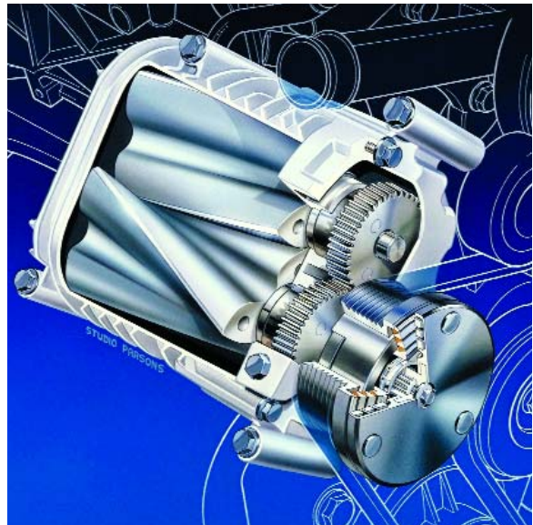
Only the supercharger on the C230 Sport Coupe and Sport Sedan use a Mercedes-Benz lubricant, Part Number A 000 989 62 01.
