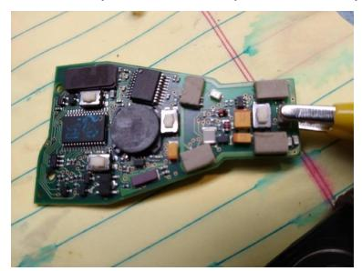
Photo is of preparation to Solder the LED back to the board.
