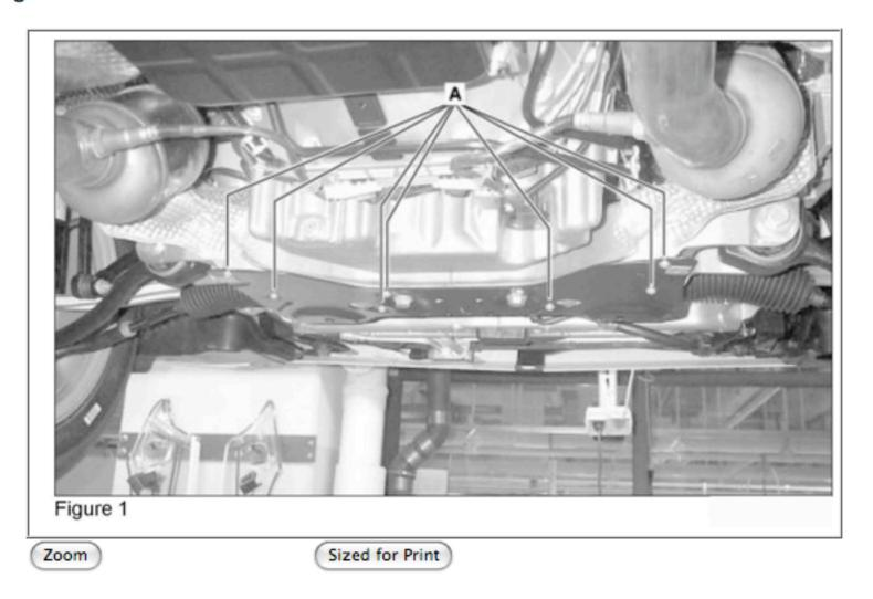
If you receive customer reports in the above model vehicles of rattling noises from front axle, the cause may be that the blind hole in the frame for mounting the stiffening plate may be too shallow (Figure 1, A). As a result, noise complaints due to the insufficient clamping force on the stiffening plate is possible. If this situation is found to exist, remove the bolts, install a 6 mm washer, reinstall the bolts and torque to a value of 12 Nm.
