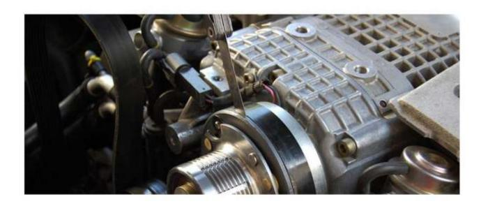
Step 9: Reverse installation. Run belt through upper idler before bolting it on. Torque upper idler bolt to 20nm. The remaining bolts can be hand tightened.
