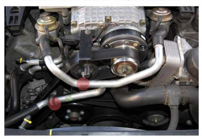
Step 2: Using the EII torx, loosen the belt by turning the tensioner counter clockwise. Slip the belt off of the middle idler.
