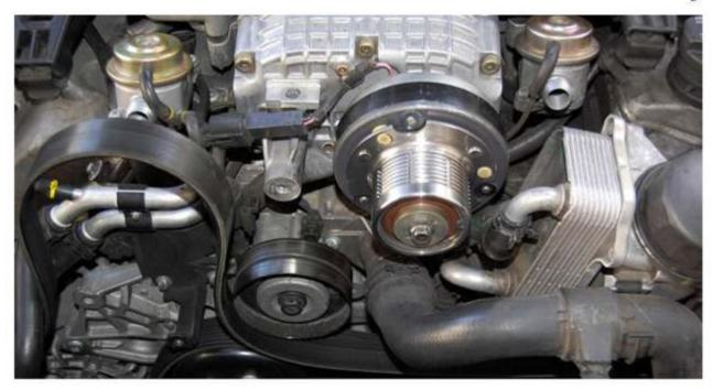
Step 4: Place rubber pad underneath SC clutch. Using the upper idler standoff as a fulcrum, place the large screwdriver or crowbar unde the pad, and apply light pressure to keep the clutch from spinning. While holding it, use the 12mm socket to loosen the sc pulley bolt.
