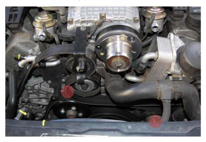
Step 3: Remove the upper idler. The bracket bolt is an E10 torx, the pulley bolt is an E12. Remove pulley and bracket.
