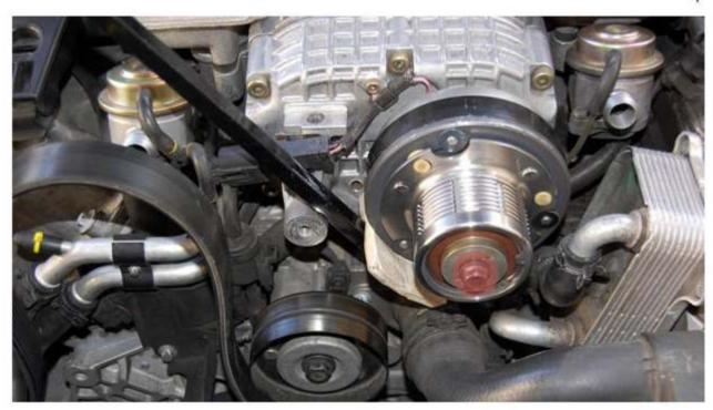
Step 5: Remove the bolt and washer from the front of the pulley.
