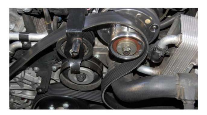
Step 10: Go over each bolt and ensure it was tightened. Turn the SC Clutch by hand, and it should spin freely. Check the belt for proper alignment on the pulleys. Once everything has been verified, start up the car. Observe the belt and pulleys, making sure there is no awkward wobbling or noise. If all looks well, go enjoy your new power.
