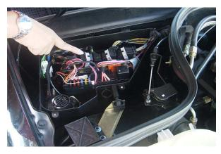
The ecu is located at the far back of the box behind the fuses.
