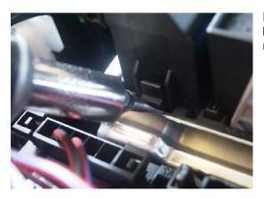
For these you will need the use of a flat head screwdriver. Push button in and remove plug.
