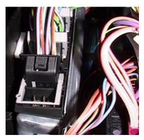
Then to release plug from ecu pull leaver down, which will lift the plug. Once the plug has been removed from the ecu it is best to lock leavers back in place as to not damage the plug.
