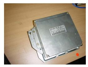
Once ECU has been removed, place on a clean workbench. The ECU is held onto a plate via four 10mm bolts. Simply undo do these bolts. The ECU required should now be free from the plate. Note the orientation of the computer on the plate before removing.
