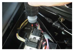
First remove the screws holding the ecu in place.
