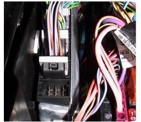
Lastly remove the three leaver plugs. To remove these press button to release leaver.
