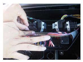
Next the two plugs on the end should be removed.
