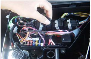
The middle plug should be removed first. Press button on side of plug and remove from ecu.
