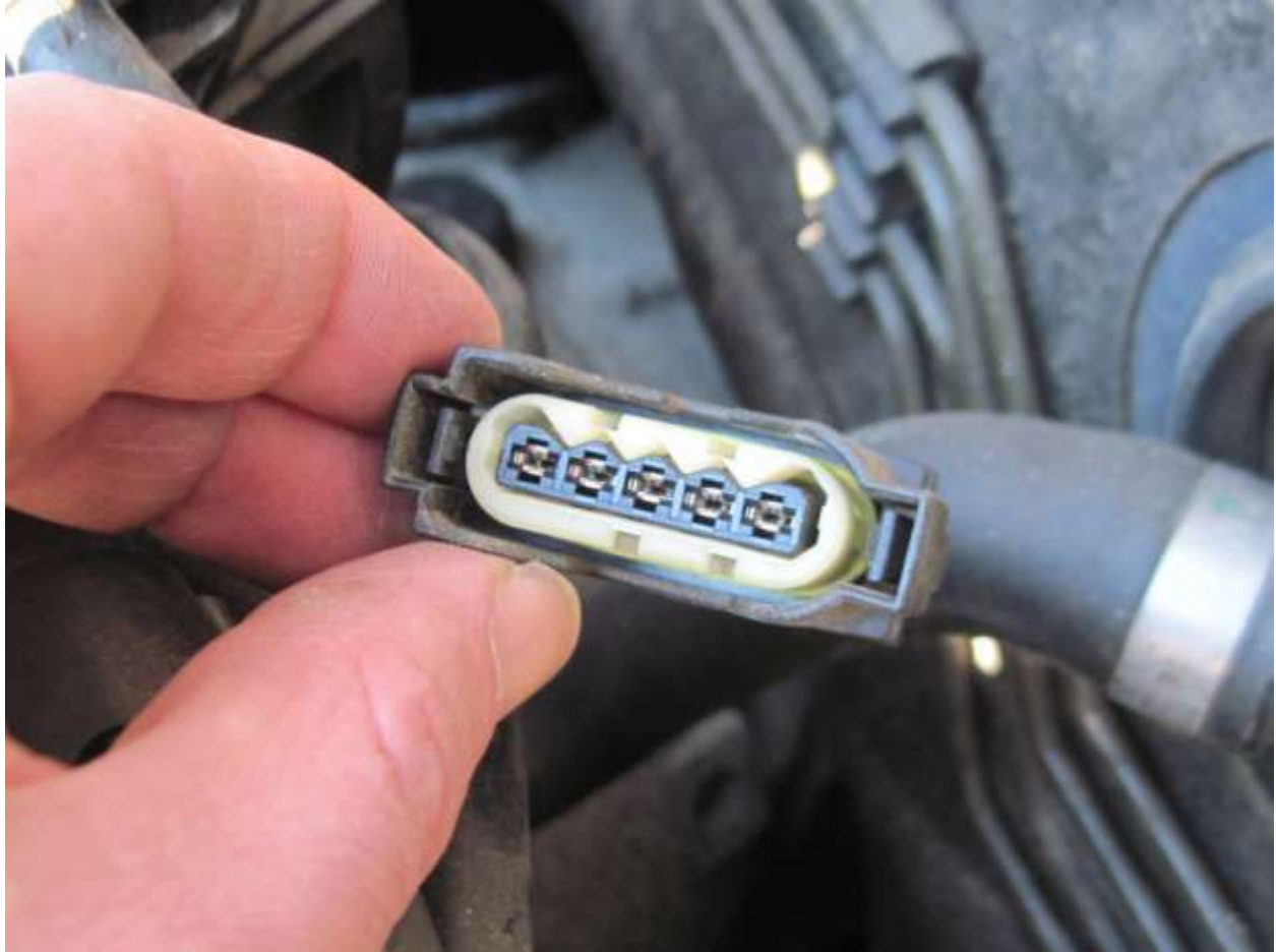
Photo 12: The electrical connector. Push it back on. You should feel it click home
