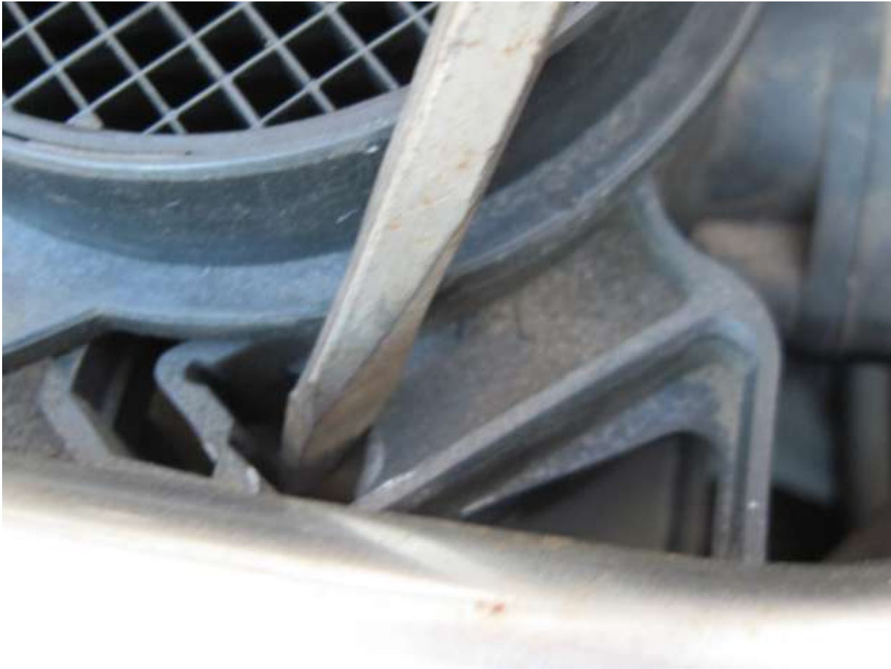
Photo 5: The Plastic Collar Again, showing how the two halves of the clip slide apart
