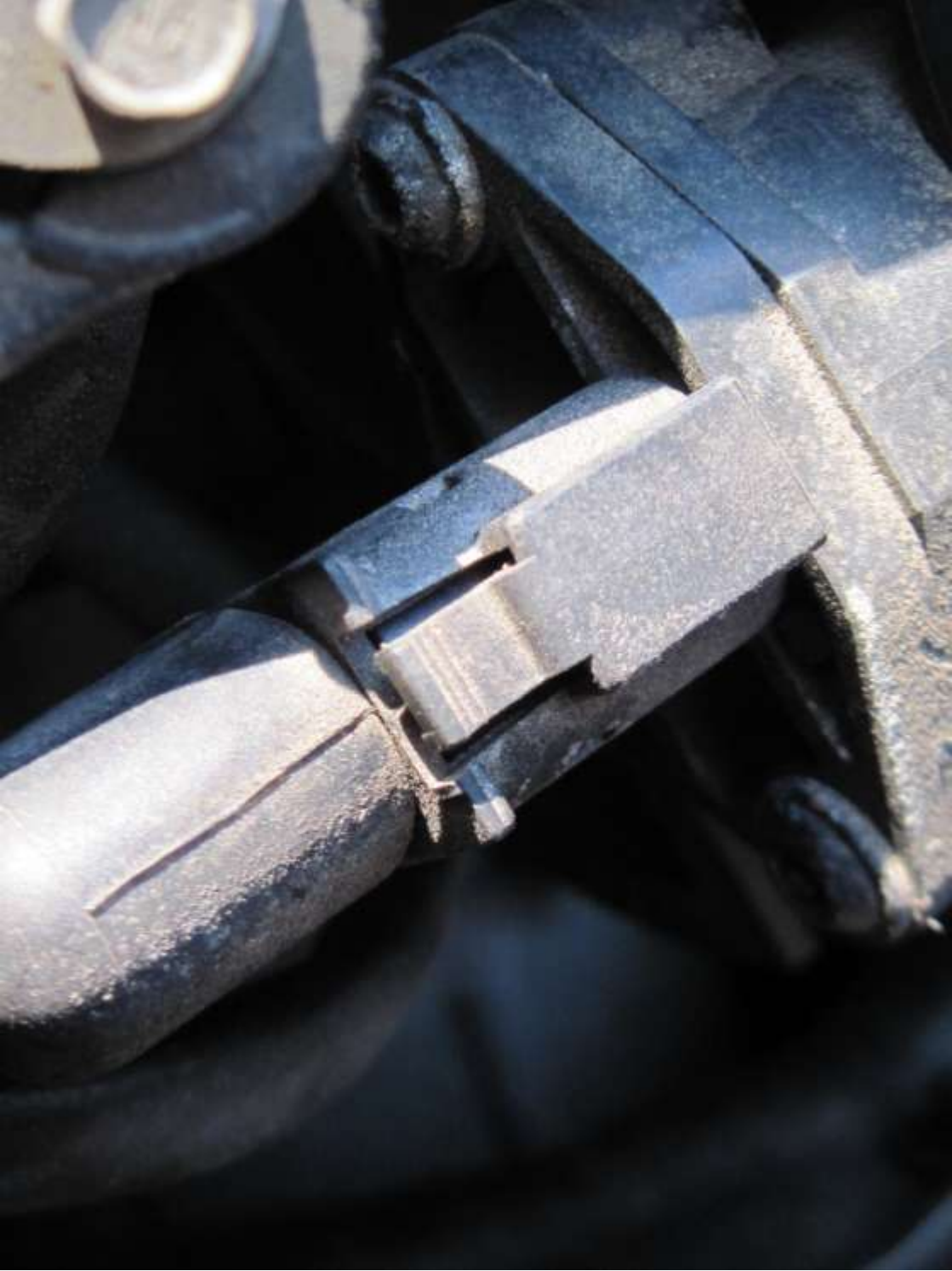
Photo 4: Another view of the electrical connector. There is a clip on the top and bottom of the connector
