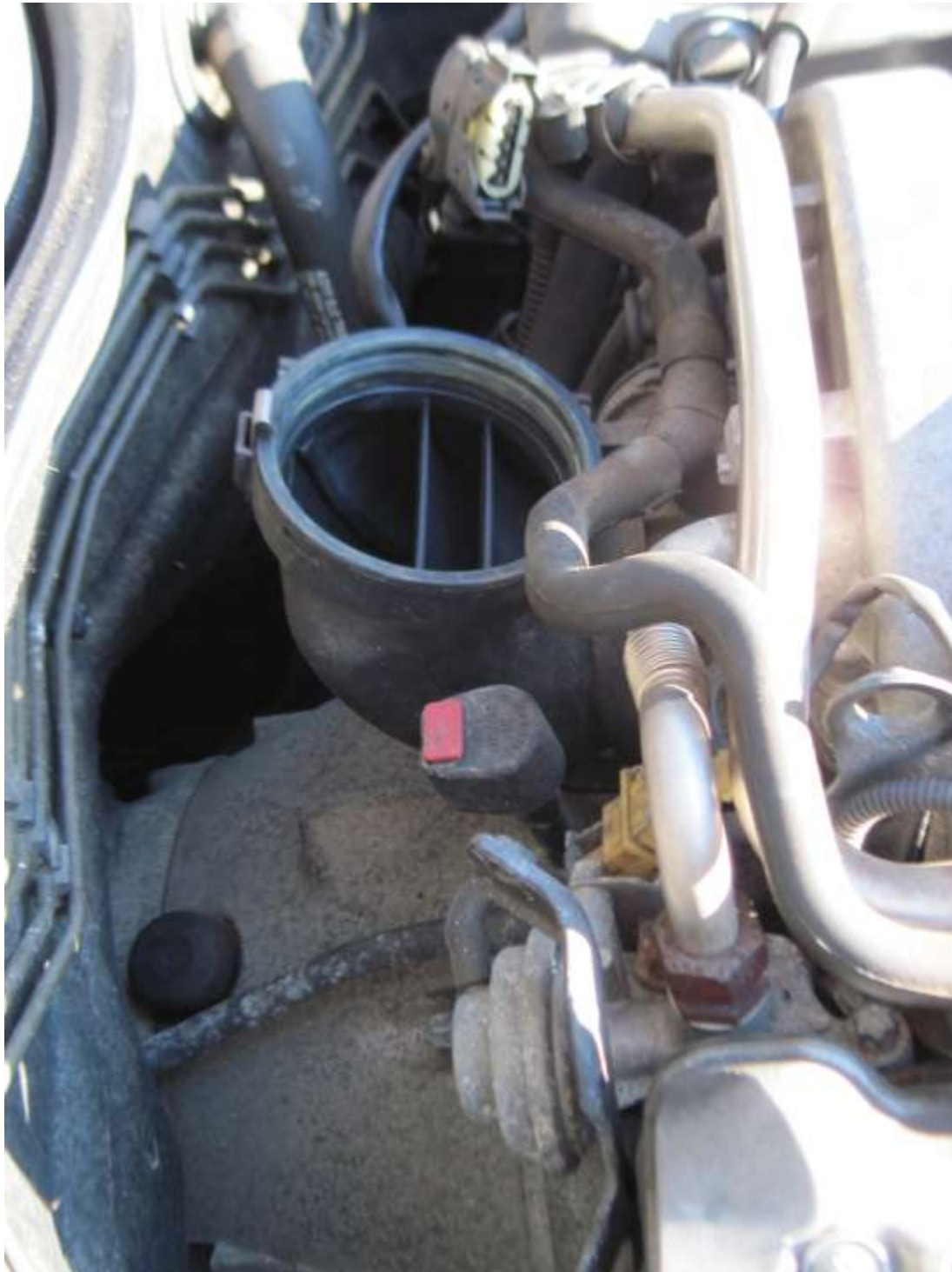
Photo 10: Another view of the engine with the MAF removed, from passenger-side this time. The MAF power-lead is to the top of frame.
