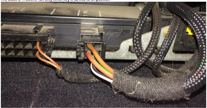
2) Remove or slide back some of the electrical tape on the wire loom.
