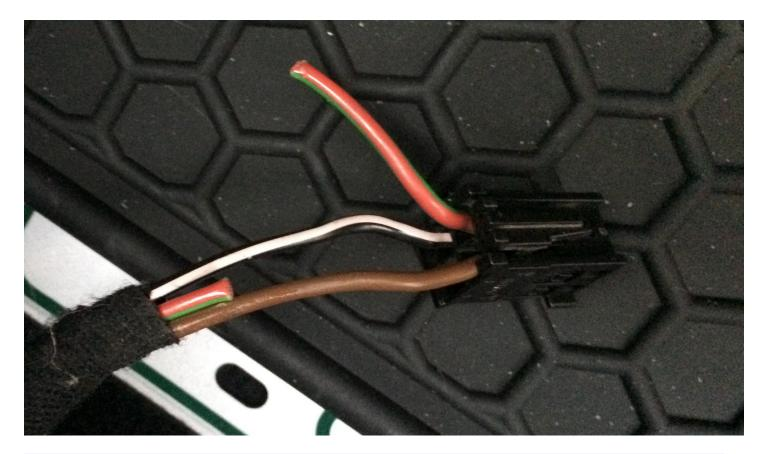
3) Cut the Red wire and Splice it with the Black wire. I removed ¼" of red wire to give more room. The black wire will provide power to the red wire only when the key is turned on.
