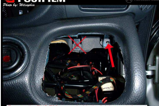
Remove the RHS T20 screws inside the lighting control panel No need to remove the LHS one (No harm if you remove it)
