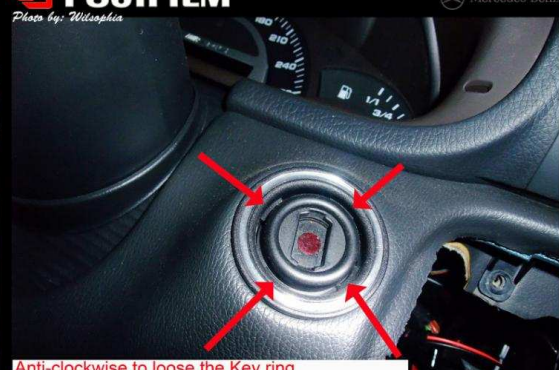
Anti-clockwise to loose the Key ring Use a small screw driver to remove the Key Ring There are 4 latches to latch the Ring
