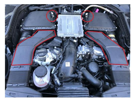
Once you remove the air duct and sensor remove the bolt holding the factory intake.
