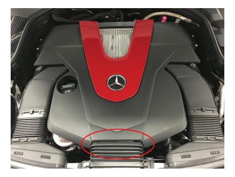
After the engine cover is removed use the small flat head again to remove the air ducts from the airbox going to the side snorkels. Once removed, unclip the sensor and twist to pull the sensor out of the air box. Push those to the side for now.
