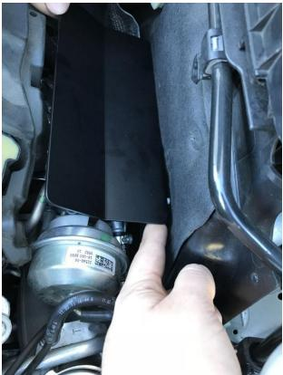
Install the BMS intake tubes to the turbo, if the factory oring is dry you can also lubricate it with engine oil or grease. Use the provided bolts to tighten the tubes down.
