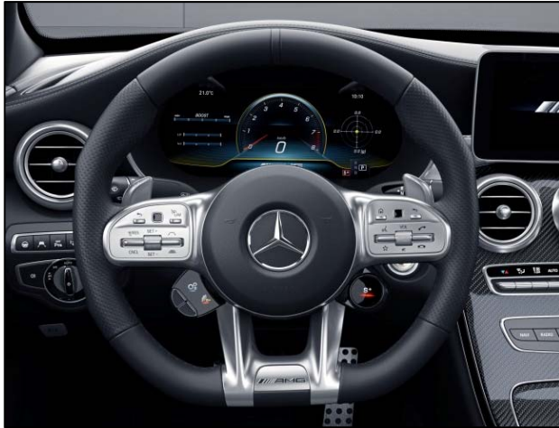
L6J - AMG Multifunctional Flat Bottom Steering Wheel in Nappa Leather with AMG DRIVE UNIT
