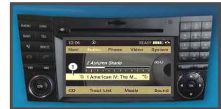
NTG 2.5 is a one piece unit with SD card slot
