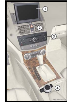
NTG 4 has controller, head unit & separate display
