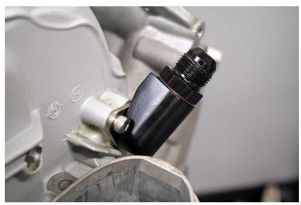
Below is a picture showing the orientation for installation on an M159 SLS Engine
