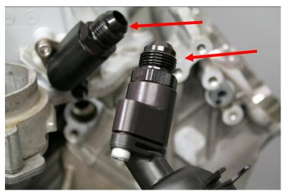
Installing billet PCV adapter onto PCV tube with a M6x16mm socket head bolt using 5mm Allen Bit and 1/4" Ratchet. (Pictured Above)
