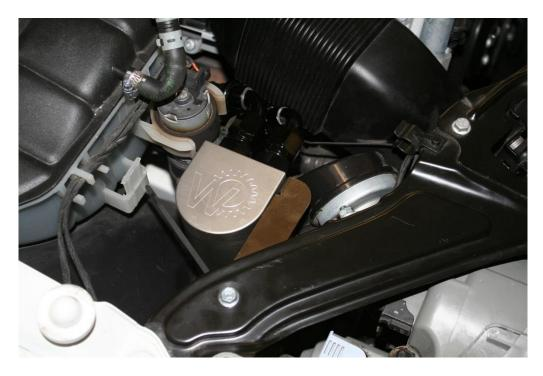
For M159 SLS AMG a hole must be cut as shown below to allow for routing of the included hoses and a special bracket is included to install the Oil / Air Separator as shown below.
