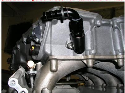
d. (Supercharged only) Sliding the PCV hold down into place and installing with a M6x10mm socket head bolt using a 5mm Allen Bit and 1/4" Ratchet.
