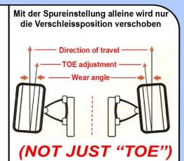
**Existing (directional adjustment)** only alters wear position but increases the overall wear rate.
