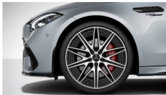
RRN - 20" AMG Twin 10-Spoke Wheel w/ Black Accents 20" R01, B51 265/35 R20 on 9.5J x 20 ET25.3 wheels (front) and 275/35 R20 tyres on 9.5J x 20 ET61.1 wheels (rear)
