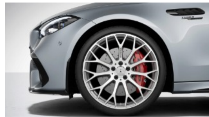
RZS - 20" AMG Forged Multispoke Y-Design Wheels Only with DA8 20" R01, B51 265/35 R20 on 9.5J x 20 ET25.3 wheels (front) and 275/35 R20 on 9.5J x 20 ET61.1 wheels (rear)
