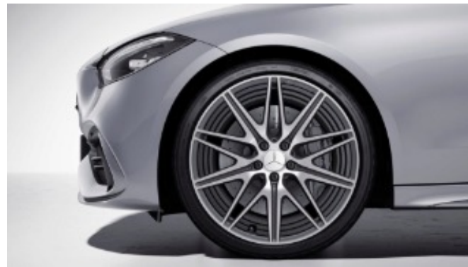
RZX - 20" AMG Split 10-Spoke Wheel 20" R01, B51 245/35 R20 on 8.0J x 20 ET43.1 (front), 265/30 R20 on 9.5J x 20 ET61.1 (rear)
