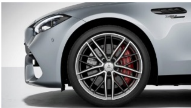
RRC - 19" AMG Twin 5-Spoke Wheel 19" R02, R66 265/40 R 19 on 9.5J x 19 ET25.1 wheels (front) and 275/40 R 19 on 9.5J x 19 ET61 wheels (rear)
