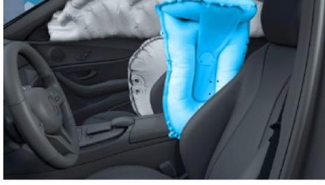
Additional airbag for increased front occupant protection in the event of a side impact
