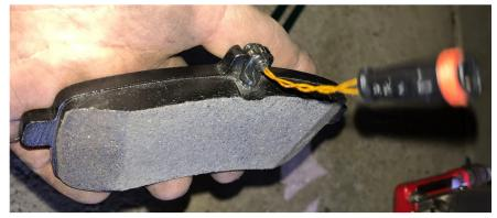
k. The new pads will come with metal clips that hold it in the position in the caliper.
