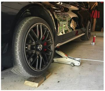
10. For fronts, jack using central jack position, install two front jack stands
