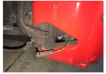
d. Remove two 13mm bolts to remove caliper, use thin wrench or pliers to hold inner bolt while loosening
