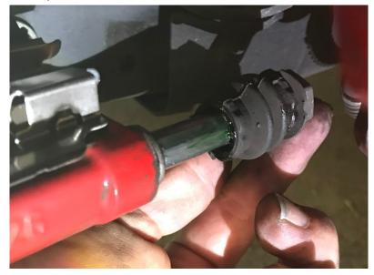
j. Install the brake pad sensor into the inner pad (passenger side only)
