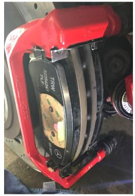
I. Compress the caliper piston all the way, checking fluid level
