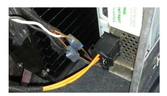
You may also connect to the CAN system at the X30/5 connector located in the foot well under the driver's seat (on left side). Connect to an empty slot on the distributor, but make sure to connect CAN-High to CAN-High and CAN-Low to CAN-Low.
