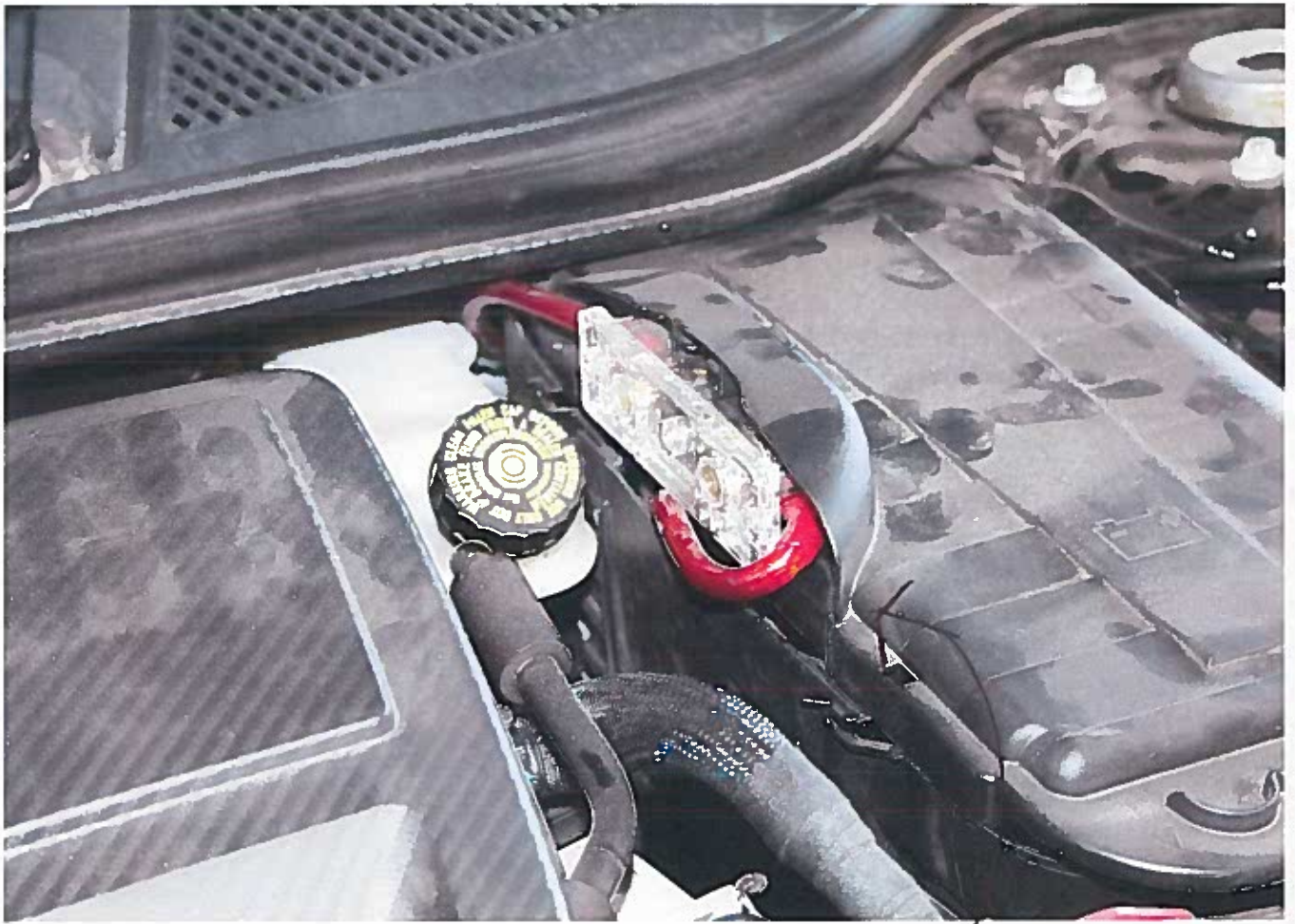
Aftermarket wiring Installed
