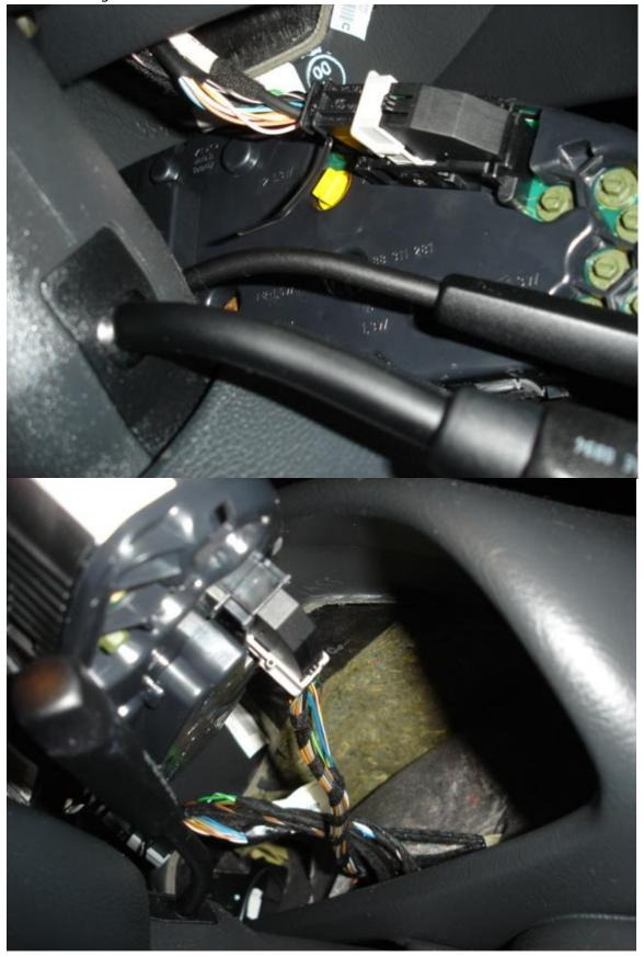
You should be able to figure that part out, but there is a small button to release the level that needs to be moved to detach the two harnesses. Once those are off you can slide the cluster away.
