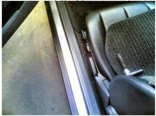
Then remove the rubber door seal (pic not shown) by gentley pulling it off from the bottom. Next undo the screw on the inside kick panel and unclip the two body to panel clips that are or were under the door seal. Pull the kick panel backwards and put to one side.
