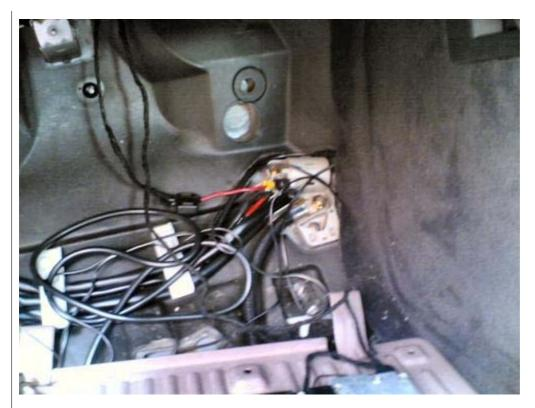
What we are looking for is the item on the right hand side. There is a black cover over a nut, remove the cover (already done in the pic). This is the main battery cable from the battery to the engine. Attach your jump lead to this nut and an earth to any solid part of the car (I used the steering box).
