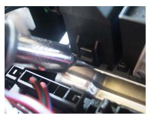
For these you will need the use of a flat head screwdriver. Push button in and remove plug.
