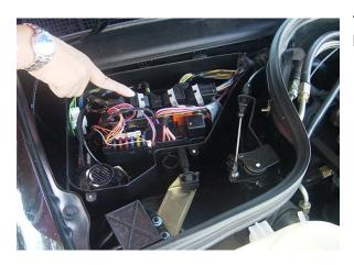
The ecu is located at the far back of the box behind the fuses.
