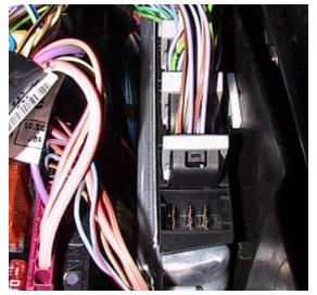
Lastly remove the three leaver plugs. To remove these press button to release leaver.
