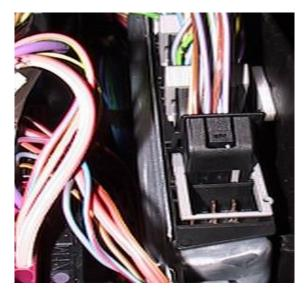
Then to release plug from ecu pull leaver down, which will lift the plug. Once the plug has been removed from the ecu it is best to lock leavers back in place as to not damage the plug.
