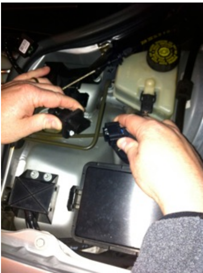
Plug vehicle's wiring harness directly into SprintBooster
