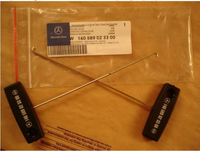
Move your steering wheel all the way out, slide the tools in at approximately 9 and 3 until they pass the little markers on the tools (as seen below).
