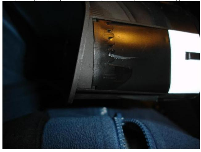
When you have a solid connection you will have to pull one side at a time to wiggle the cluster out, but before then and this might scare you, but you have to give that first hard tug to get the unit moving. Once it's looses then easy does it by wiggling it out.
