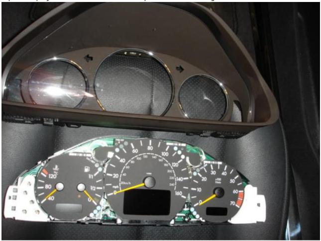
I worked on the two small rings first using the middle opening to place the rings through as it's larger [;)] Just make sure that they are centered as much as possible.
