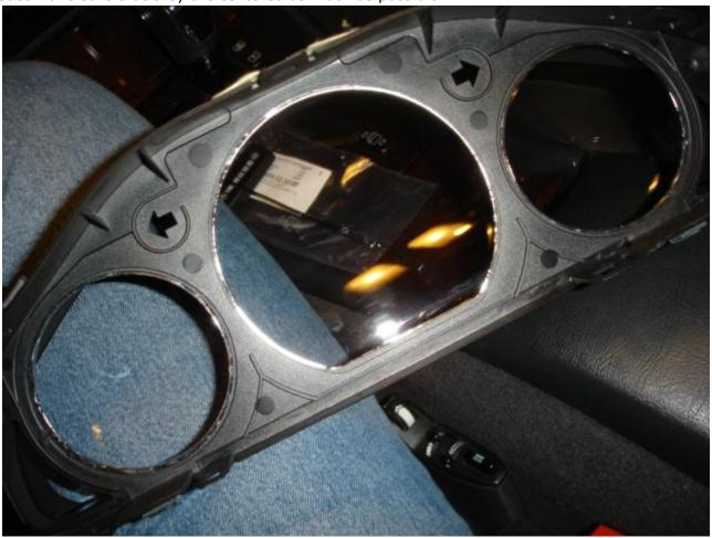
Once the rings are all on you can put the cluster back together. There are two small plastic pieces that by now have fallen off of the cluster don't worry, but you can't put them back before you put the two pieces of the cluster back together, well almost together. You should be able to figure this out if you study were the pieces fit and the slots that are on one of the two halves of the cluster.
