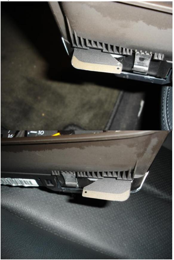
Be careful here because this is where things get tricky. Once back together slide the cluster back behind your steering wheel and reconnect the wiring harnesses, before sliding the cluster back in place you key into the ignition to make sure all the lights and LEDs come on.
