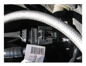
5. Disconnect the electrical connectors by pulling on the "T" handles at the front and rear of the connectors. Also unscrew the small bracket that they are zipped tied to or cut the zip tie.
