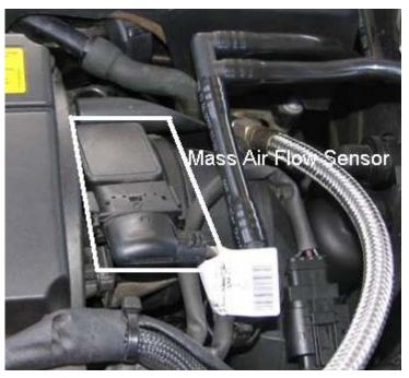
To get to the Mass Airflow sensor you need to remove the air filter box. It is held in place by two bolts toward the rear and two rubber bushings in front. Other items that are attached to it are a flex duct going to the supercharger, various electrical connectors, crankcase ventilation tube and also a vacuum line that needs to be disconnected for clearance.
