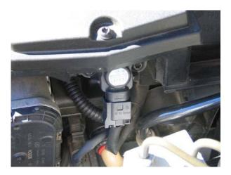
7. Disconnect the crankcase ventilation tube.
