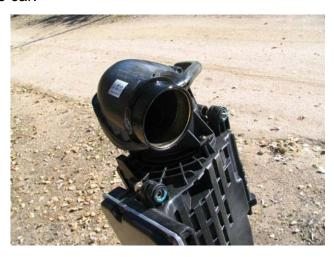
12. This is the end of the air box with the MAF sensor. Three screws hold it in.
