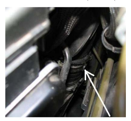
10. Everything is now disconnected that needs to be, it takes a bit of pushing aft and twisting towards the left to get it out. The filter box has two pins at the forward end that holds it in place with rubber bushings. The main thing is to keep all the connectors and hoses out of the way and it will come out with a bit of effort. You can actually see the intake manifold now.
