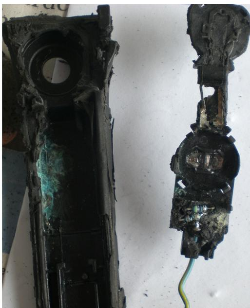
*You can see the 2 resistors in the above photo. The top one is 470 ohms and the lower one is 300 ohms.*
