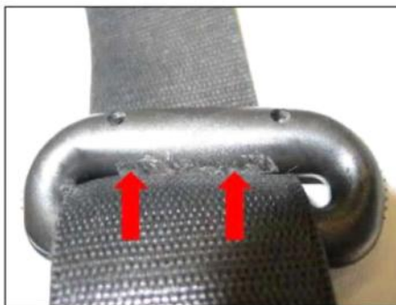
Figure 2 Deposits on belt guide
