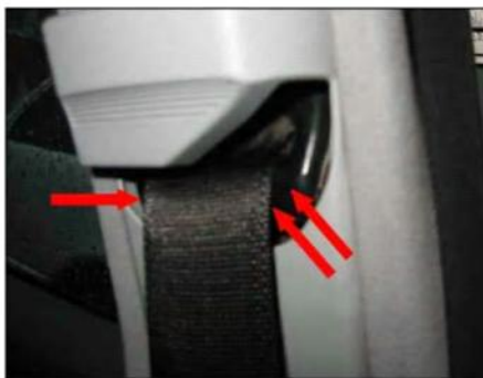
Figure 1 Area of belt guide to be cleaned
