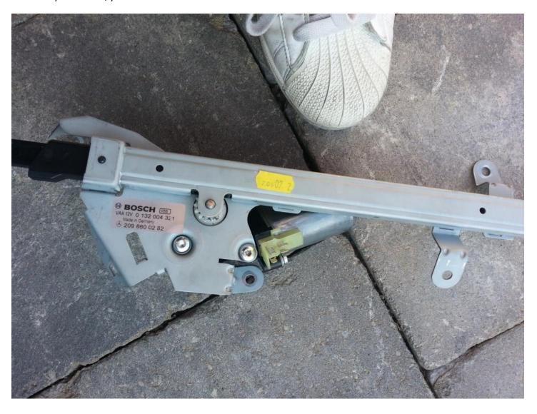
10. The culprit in my case. Note a tooth is missing from the sprocket. The whole thing is held on by three clips which you can just pry off. Open it up and replace the sprocket if that's what you need to do. Or just replace the whole motor.
