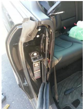
4. About ¾ of the way down the door there is a tiny little plastic tab thing. It has a hole in it. You need to use some needle nose pliers or something to grab it and pull it out. That will release the clips.
