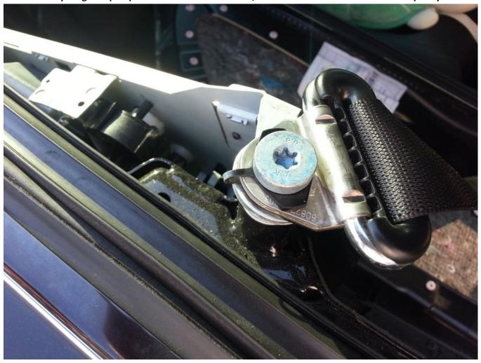
8. The assembly is held on by two 10mm nuts. Remove them. Don't drop anything – if you do, solid chance the nut ends up in the deep recesses of the door panel that would be a huge pain to get to...imagine years of endless rattling. Be cautious. Also, remove the wiring molex thing. A screwdriver (precision type) helps here.
