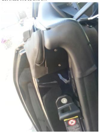
3. And remove the rubber weather stripping. Two pieces, one smallish rubbery "elbow" piece and the big weatherstriping piece that goes down to the sill.
