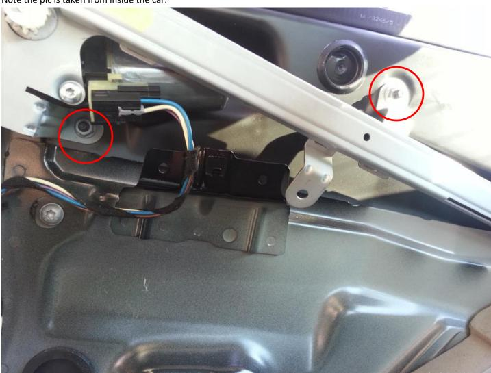
9. The assembly comes right out now. If you haven't already, remove the plastic arm by pulling SLOWLY. You will be forcing the sprocket to drive the worm gear of the motor, so don't yank like it's the apocalypse. If you need to, you can remove the motor with a T20. The two screws below.
