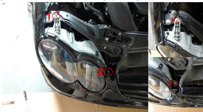
Step 12: With all the three Headlight mounting screws removed, you will be able to remove your Headlight from your car. When removing your Headlights, please be mindful of where the adapters are and unplug them as you pull your Headlights out of your car's frame.
