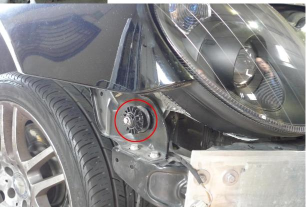
Step 11: Remove two 8mm screws on top of the Headlight by unscrewing them with an 8mm socket.
