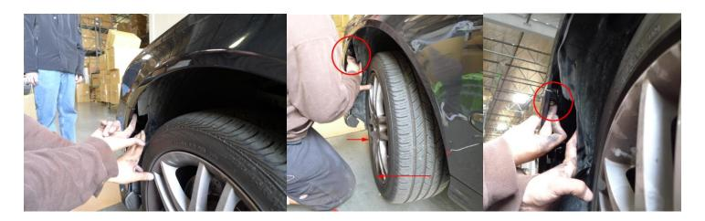
**Step 4**: Remove "Mud-guard" by unscrewing <u>three</u> <u>8mm</u> screws that is similar to the one that was found in the tire-well from *Step 3*.
