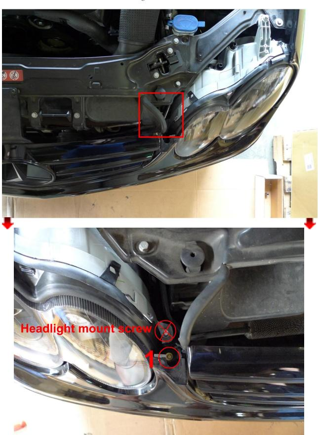
**Step 8**: After you have removed screws/clips from the top-side of your car, you must unscrew the 8mm screws that are hidden below and behind your car's Bumper and Grille. There will be an opening for your screwdriver on each corner. *Please be mindful of where your unloosened screws are. Try not to let the unloosened screw drop into your car's interior bumper lip.*
