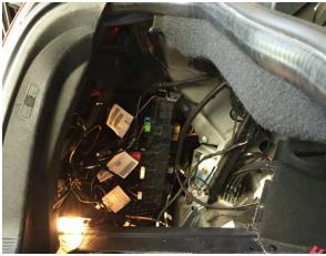
b. The Tel module needs to be inserted between the "Sound" and the "SDARS" so that the original connection was: SDARS-IN connected to Sound-Out, and UHI-In connected to UHI-Out.
