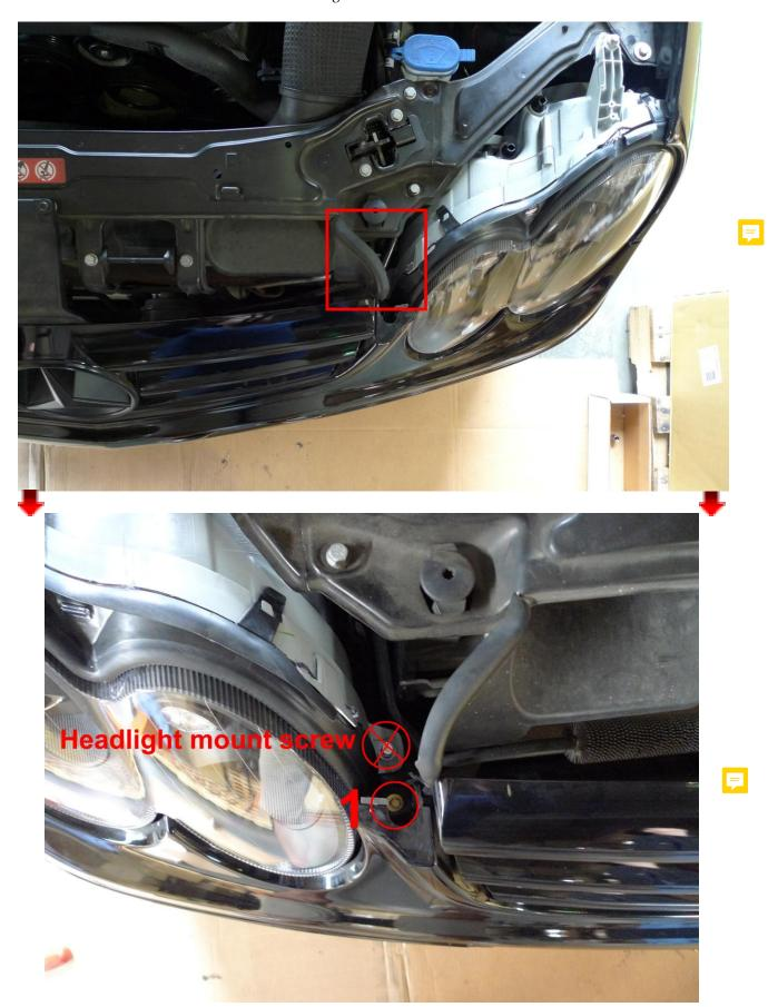
**Step 8**: After you have removed screws/clips from the top-side of your car, you must unscrew the 8mm screws that are hidden below and behind your car's Bumper and Grille. There will be an opening for your screwdriver on each corner. *Please be mindful of where your unloosened screws are. Try not to let the unloosened screw drop into your car's interior bumper lip.*
