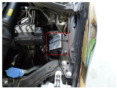
**Step 15**: After you have properly secured "Headlights & *HID Ballast mounting bracket*" to your car, you should test the headlights. Test all features BEFORE you put re-install everything back to the car.
