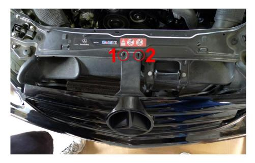
**Step 7**: Next, you must unscrew the 8mm screws that is in between your Headlight and Grille. There is one 8mm screw on each side of the Grille. *Please be sure to not confuse the Headlight mount screw with the 8mm screw that is in between the Grille and the Headlight.*
