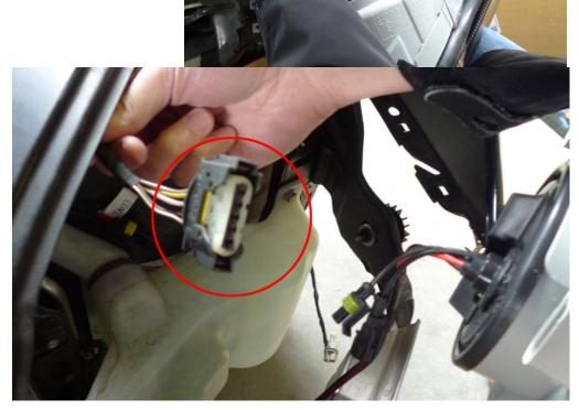
**Step 13**: If you have purchased the headlight without Xenon HID system included, simply reverse the process above to install the new headlight in. If you have purchased the version with Xenon HID included, it is the same exact procedure except you need to follow the below Step 14 to secure the ballast in a proper location. Disregard Step 14 if you did not purchase the headlight with Xenon HID included.
