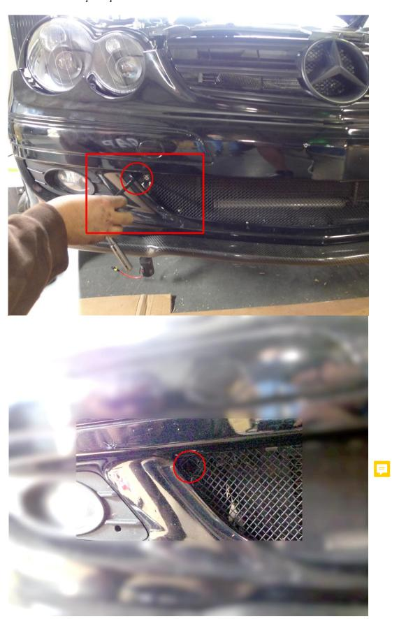
**Step 9**: Next, you will need to remove six clips underneath your car's bumper. Once you have done this, you should be able to remove your car's bumper. Slowly and carefully, from one fender-end of your bumper to the other, pull the bumper off of your car's frame.
