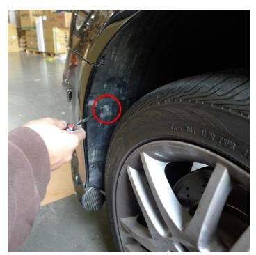
**Step 2**: Then unscrew and remove the <u>10mm</u> screw inside the tire-well with a 10mm socket. The 10mm screw is located to the lower right of "clip #2" in the picture example from *Step 2*. Do this for each front-side tire-well.
