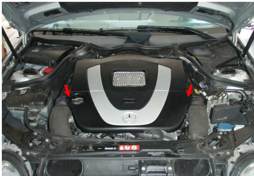
Figure 13 – Re-attach front engine cover
