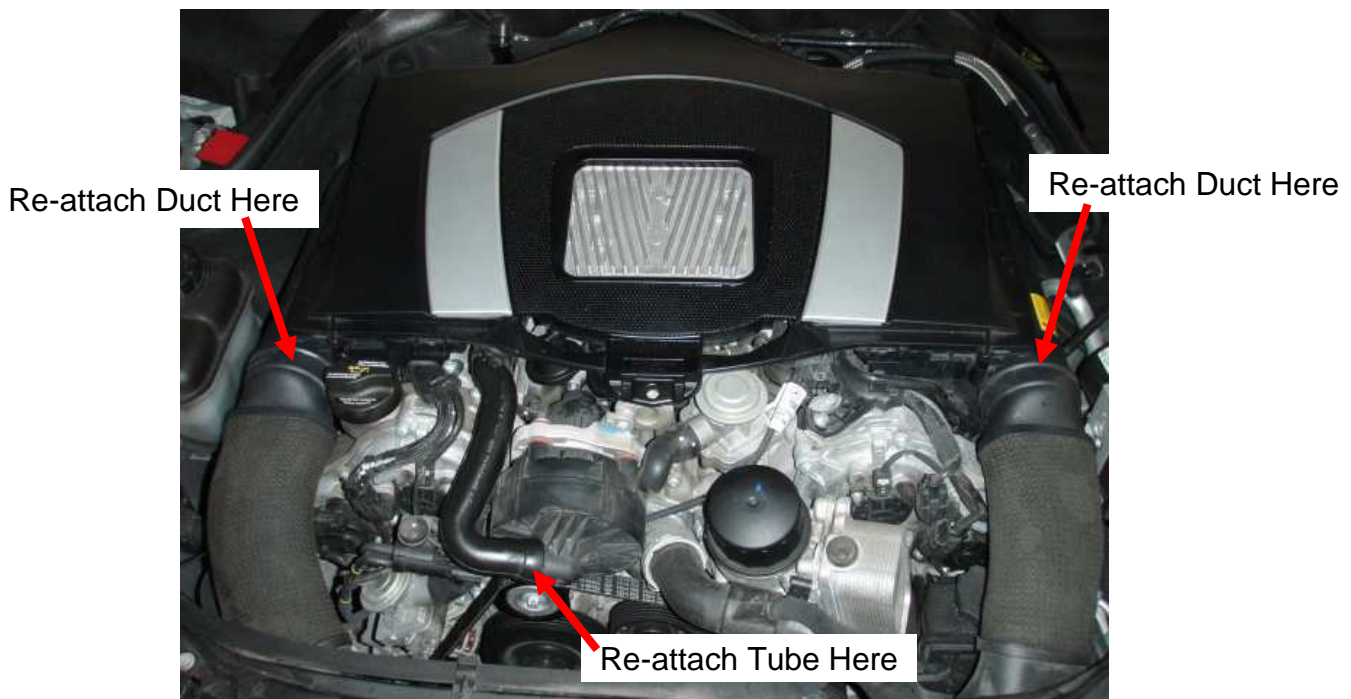
Figure 12 – Installing tube and ducts.
