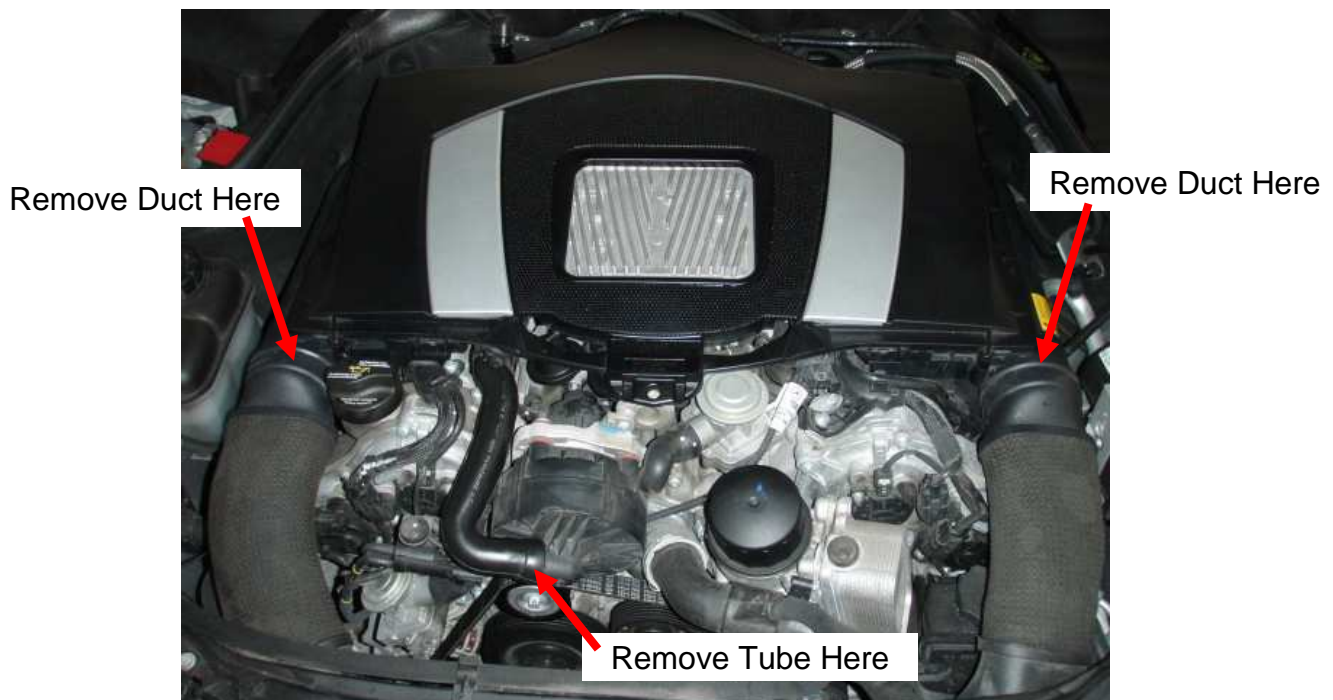
Figure 2 – Removing the intake air box
