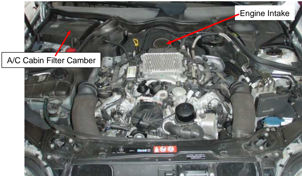
Figure 11 – Engine Bay with front cover and intake air box removed.
