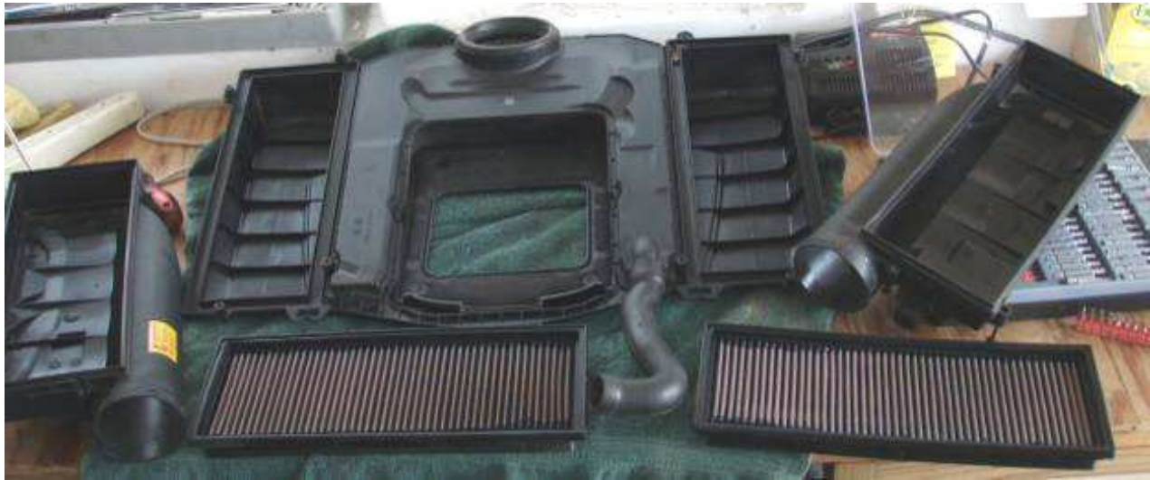
Figure 7 – Air filter removed from the air filter chambers and intake air box.
