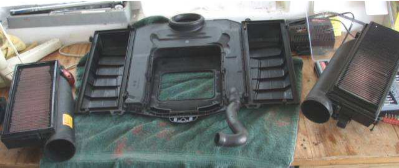
Figure 6 – Air filter chambers removed from intake air box (look how dirty the filters are).
