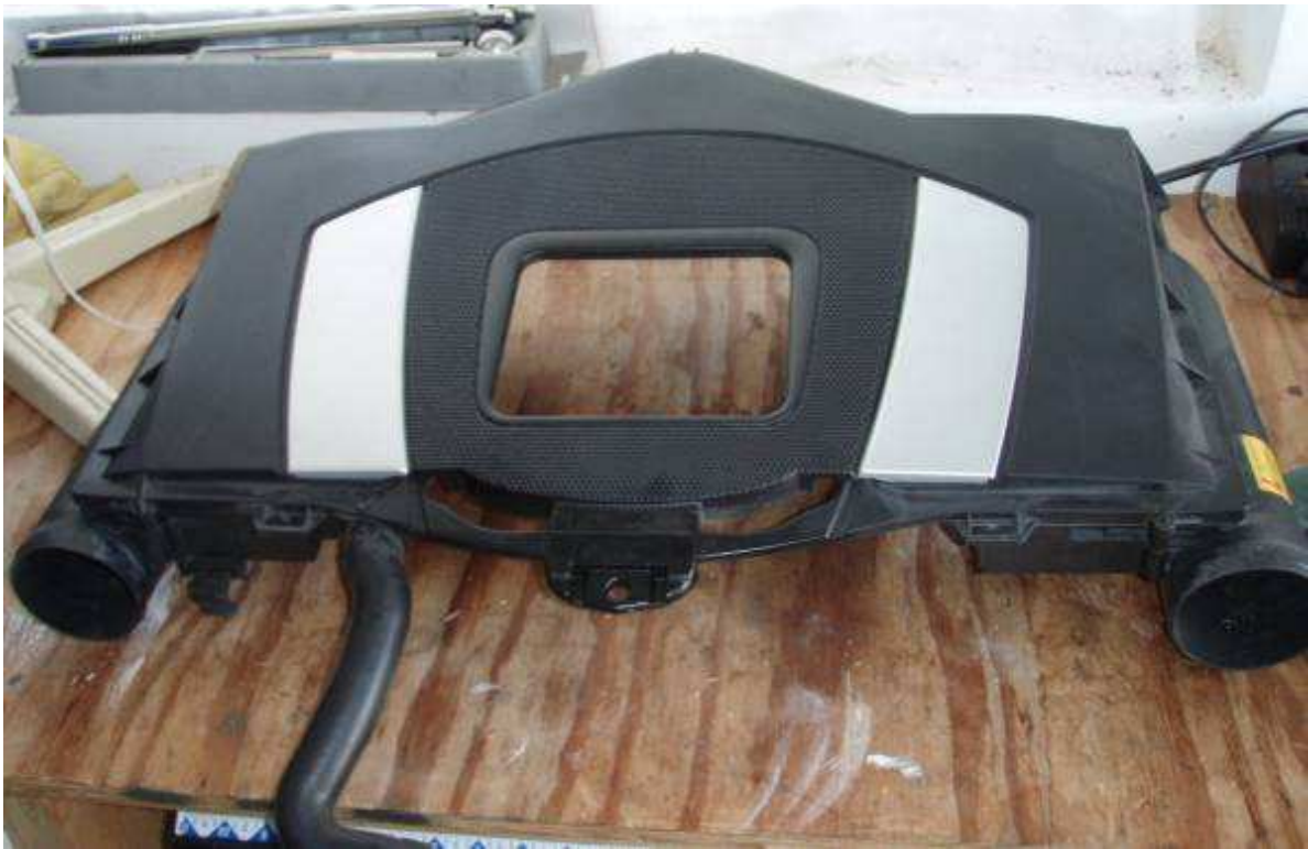
Figure 4 – Intake air box removed from engine bay
