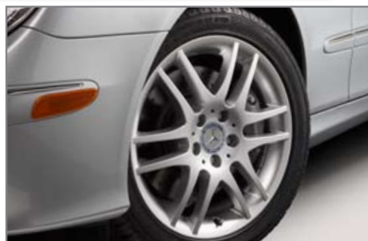
17" Staggered Width 6-Split-Spoke Wheel with Lowered Sport Suspension
