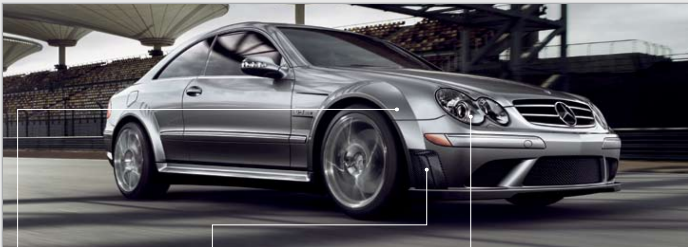
Carbon fiber re-inforced plastic front apron with carbon fiber air outlets in front of each wheel
