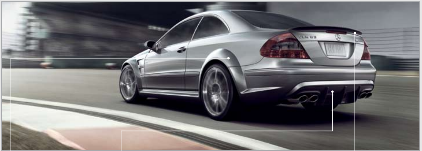
Carbon fiber re-inforced plastic flared fenders and rear apron
